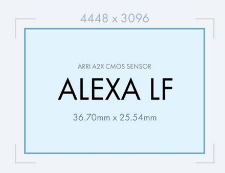
The Alexa LF sensor is roughly twice the size of the Alexa sensor. It has a similar image area to an 8-perf 35mm negative.
