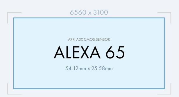
The largest sensor of the Alexa family, the Alexa 65 sensor is roughly equivalent to three regular Alexa sensors aligned next to one another.
