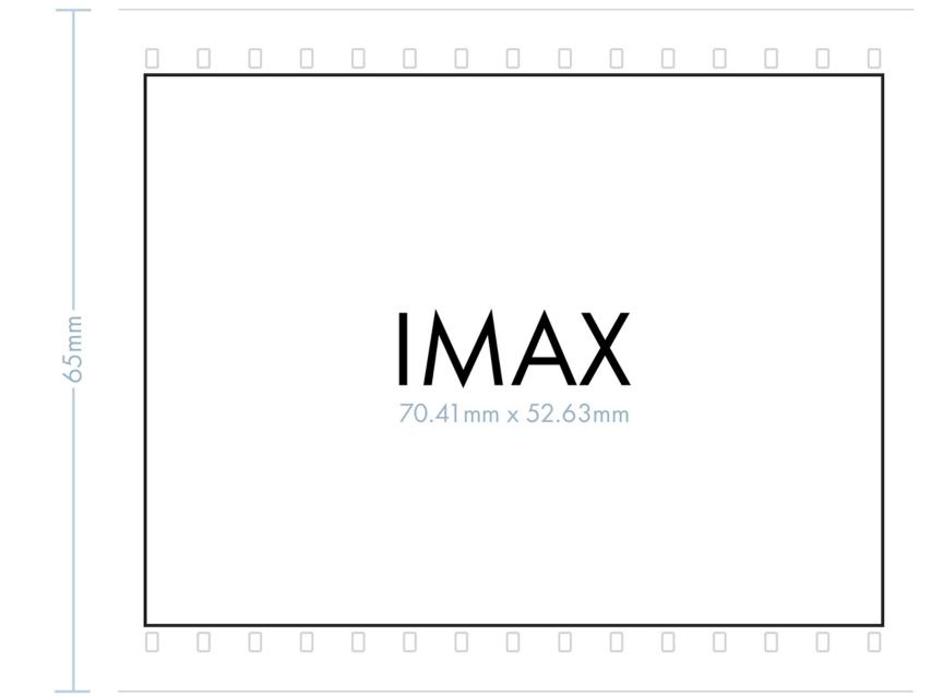
The IMAX camera aperture is a 15-perf image area on 65mm film, shot horizontally. Also known as 15/70 format. IMAX is projected on 70mm print films.
