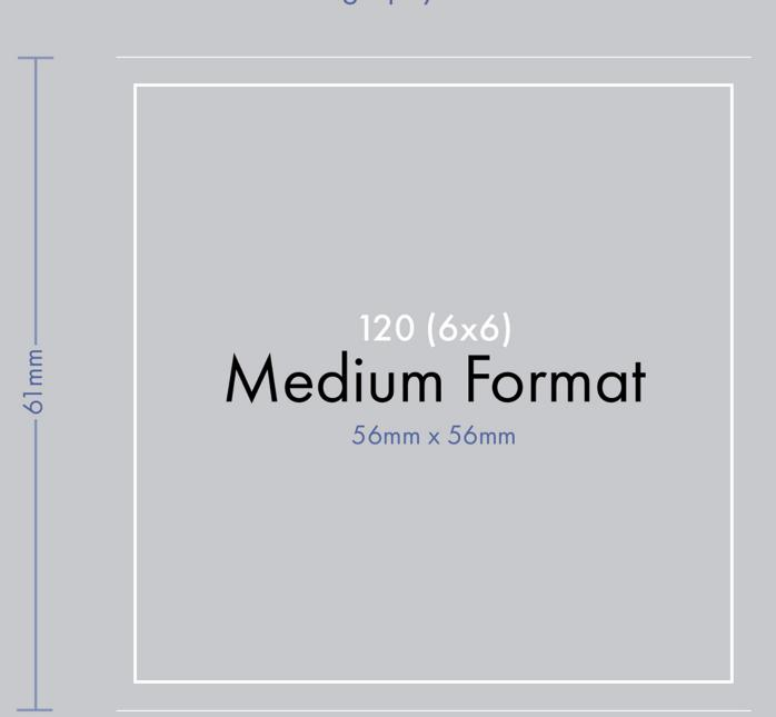
120 Medium format still photography uses roll film without perforations. Available in different formats, most commonly 6x4.5, 6x6, 6x7 or 6x9.
