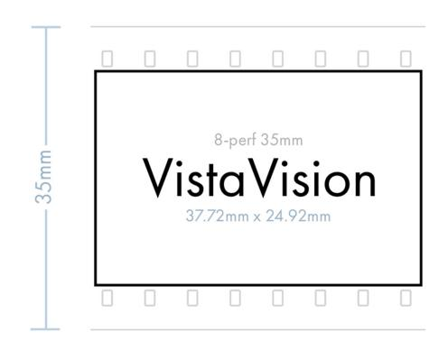
VistaVision uses 35mm film at 8 perforation per frame. The film runs horizontally over the gate, like on IMAX.
