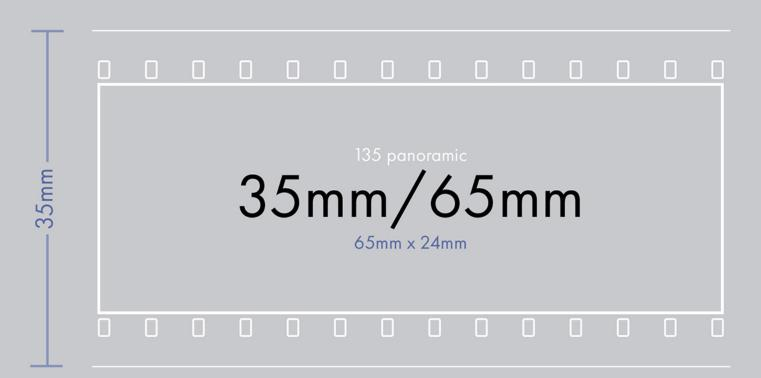
This less common format is possible with regular 135 film by using cameras such as the Hasselblad XPAN or some medium format cameras coupled with an adaptor.
