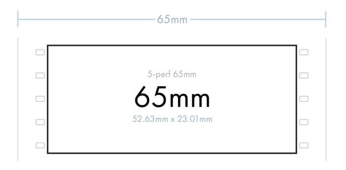
5-perf 65mm formats uses the same film as IMAX. However, the classic orientation and wider aspect ratio results in smaller frames with a three times larger shooting ratio.
