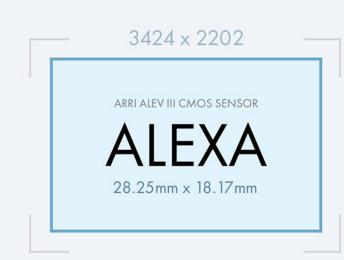
The full Alexa sensor accessible by shooting Open Gate. The Alexa Mini and Amira use the same sensor. The majority of shooting options uses a cropped section of the camera sensor. Amira only allows cropped modes.
